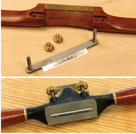
Material difference. The difference is more than material between a wood-bodied and metal-bodied spokeshave. Notice the difference in cutting angles – when assembled, the wooden-body’s blade is close to parallel with the sole.
