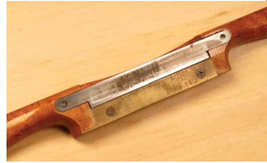
Hollow grind. Cutters with hollow-ground bottoms make sharpening fast – only two narrow strips of metal have to be dressed rather than the entire blade surface.
