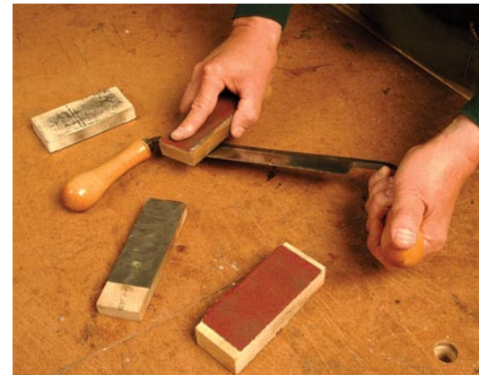
Dress all surfaces. Make sure you dress the entire curve on the front of the blade to maintain its original shape. Don't just dress the edge, or the angle will gradually increase.
