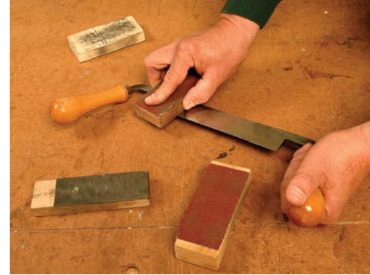
Flat bottom. Although the blade should be ground with a knife edge, the back of the drawknife should be flat, like a chisel.
