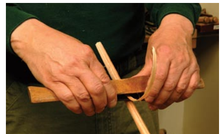
Proper stroke. A spokeshave is, 90 percent of the time, used on the push stroke. However, if you have a straight-grained workpiece such as a chair spindle, it can be pulled effectively.
