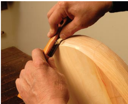
In a pinch. The handles suggest that one grip the shave by the handles. However, more control is gained by pinching it in the center.
