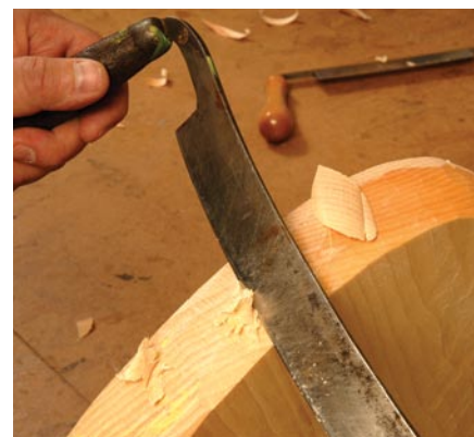
Unclean cut. If you hold the knife upside down, the angle of the blade is higher and you're likely to get a crumpled shaving and rough surface.
