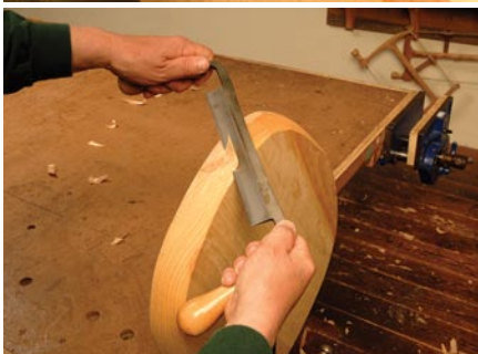
Get a grip. There are many different ways to grip a drawknife, depending on your goal. How you hold the knife is a function of your work.
